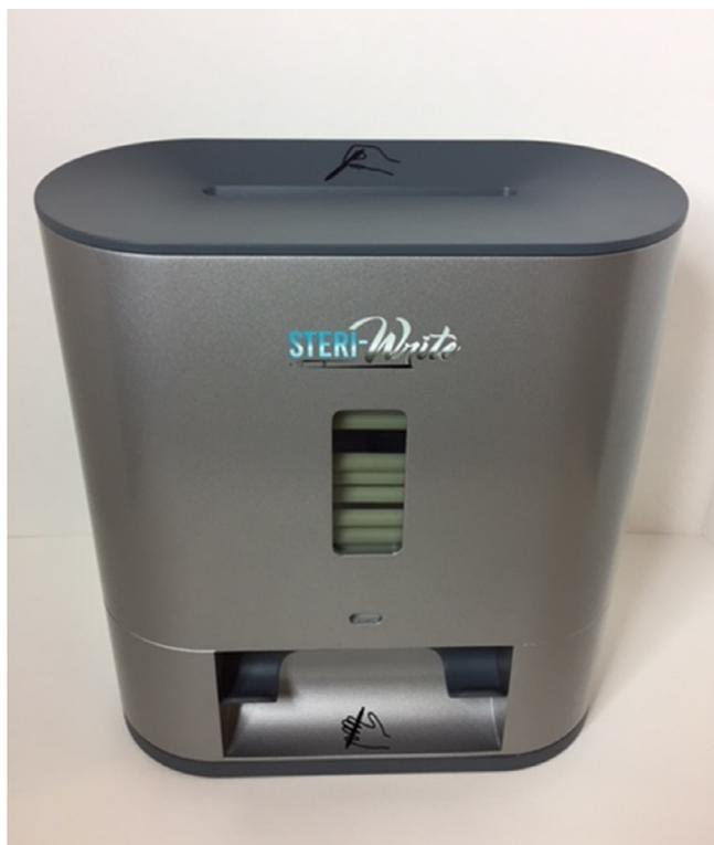
**Fig 1.** Steri-Write device. Pens placed in the top of the device are automatically loaded onto a conveyer system that rotates the pens to provide ultraviolet-C exposure to all sides for a total exposure time of 30 or 90 seconds. After cycle completion, decontaminated pens are dispensed at the base of the device.
